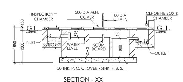
THE DEPTH OF SEPTIC TANK AND SEMI UNDER GROUND WATER RESERVOIR SHALL NOT EXCEED THE DEPTH OF FOUNDATIONOF BUILDING, PRECAUTIONARY MEASURE WILL BE TAKEN AT THE TIME OF CONSTRUCTION. OF BUILDING AND SEPTIC TANK AND SEMI UNDER GROUND WATER RESERVOIR AND ADJOINING BUILDING
